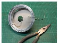
When using a wire spool, this is how they dispense wire without binding.
